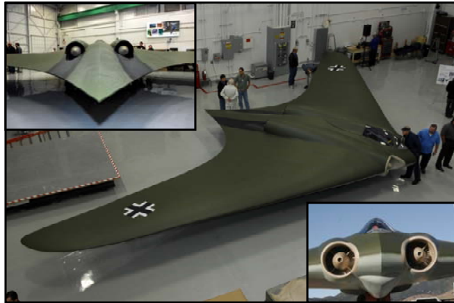
Figure 1. Full Scale Ho-229 RCS Pole Model
